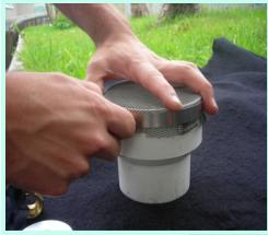
Insert the PVC reducer into the 3 inch hole in the lid of the barrel.
